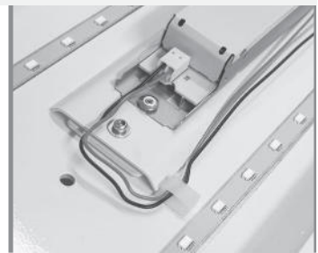
ASA - TREIBER MIT LED MODULEN / ASA - DRIVER WITH LED MODULES
